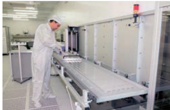
Vacuum machine for application of chromium layers
