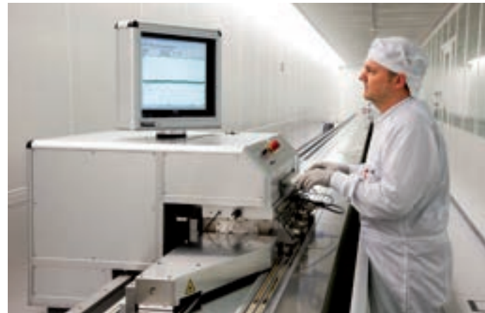
30 m long measuring machine for scale tapes
