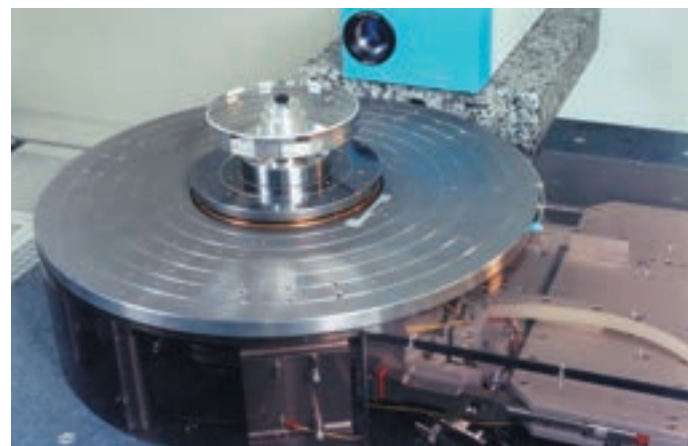
Angle comparator, measuring step approx. 0.001°
